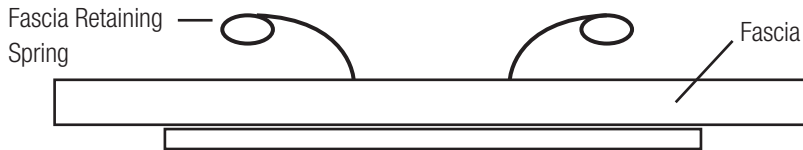
Fig. 3: Fascia retaining springs side view
