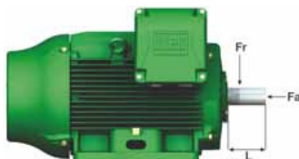
Figure 20 - Radial and axial thrust on motor shaft
