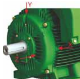
Figure 6 - Flat surfaces for vibration checking on the DE side (frames 225 to 355)
