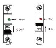
WARNING: If MCB trips it maybe caused by either, overload, short circuit or earth leakage. The installation should be checked before resetting MCB.
